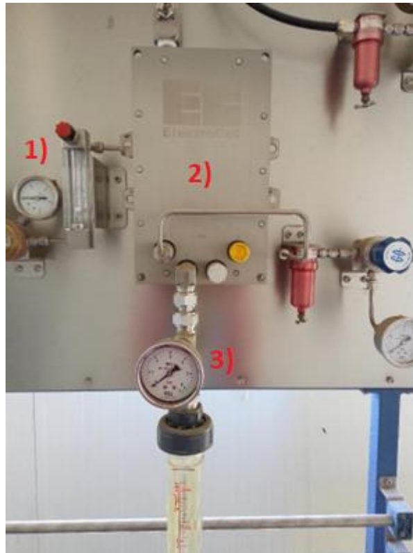
Figure III.16: The EO cell set-up, with 1) the air-inlet and pressure meter, 2) the EO cell, 3) the water-inlet and pressure meter.
