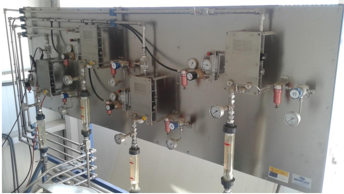
Figure III.14 Error! No bookmark name given.: Photo of the system wall containing four cells for EO treatment of water.
