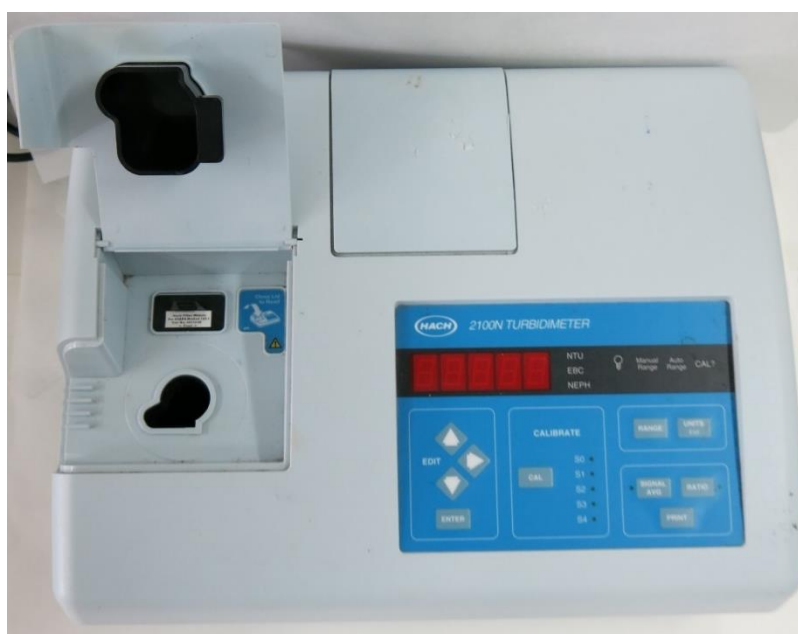
Figure III.3: Turbidity meter used in the TSA lab at the PSA, of the type HACH 2100N.
