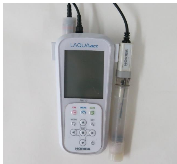
Figure III.2: The mobile pH meter used in the TSA lab at the PSA.
