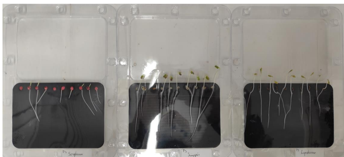
Figure III.9: The translucent plastic cassettes containing the black colored foam pad and the germinated seeds of the three plant species Sorghum saccharatum (left), Sinapis alba (middle), and Lepidium sativum (right).
